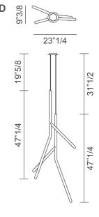
**A,B:** Lighting system with LED COB 13W 1200LM 3000°K, not dimmable. Provided with suspension cable up to 1,5mt.
