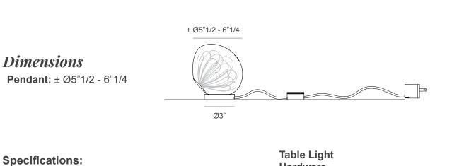
Glass Color: White Lamp: 1.5W LED, 2500K, 130lm Base: Ø3" Cable length: 90"1/8 black flexible cord Finish: Unlacquered brass base and dial control Materials: Glass, brass, electrical components Power Supply: Integral, dial control with build-in dimmer Input 100-240V, 0.5A 50-60Hz Output 12V Ta 25°C Dimming: Built-in dimmer ONLY Environment: Indoor, dry location. IP30
