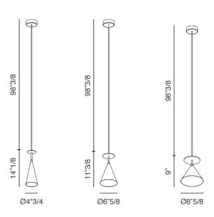
ABC Single Suspension Lamp A:  $\emptyset$ 4"3/4 x 14"1/8H ABC Single Suspension Lamp B:  $\emptyset$ 6"5/8 x 11"3/8H ABC Single Suspension Lamp C:  $\emptyset$ 8"5/8 x 9"H
