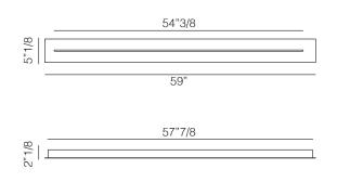
Lights Tracks are only for Sky-Fall pendants. Each pendant should be separated from the Canopy and installed on the Track. Each pendant should be installed on the Track using the driver removed from the Original Canopy.
