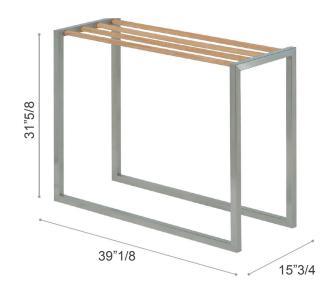
Brushed hairline finished **Stainless Steel**, type AISI304 18/08 with 18% chromium and 8% nickel. Wall thickness of the Stainless Steel tubes: 1/16". The electropolishing treatment of the frame is recommended to be used in a corrosive environment.
